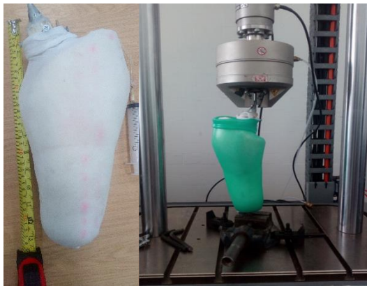
Figure 7: Image from the left - Stump model, showing the syringe controlling the volume. Image from the right – Experimental set up with liner inserted in the stump and the Instron Machine attached.
